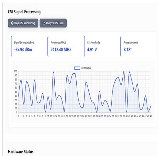
Fig 4: Flask Admin Dashboard showing real-time CSI amplitude variations across all subcarriers.
